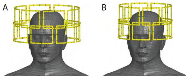
Figure 4.3.5.1 Array geometry setup: (A)  $\varnothing 280$  mm and the head displacement 12 mm, (B)  $\varnothing 230$  mm and the head displacement 27 mm. Only radiative elements and human model are shown.
