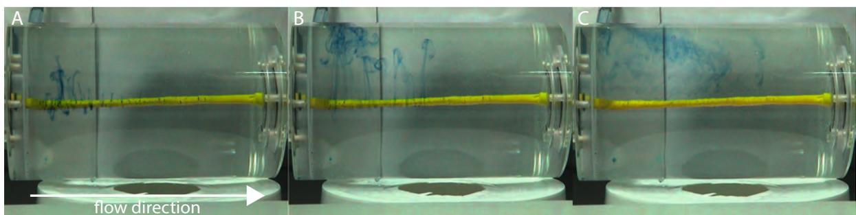
Figure 4.1.9 Experimental model of a single capillary using ink as a tracer at (A)  $t = 0.5$  s, (B)  $t = 3$  s and (C)  $t = 10$  s.
