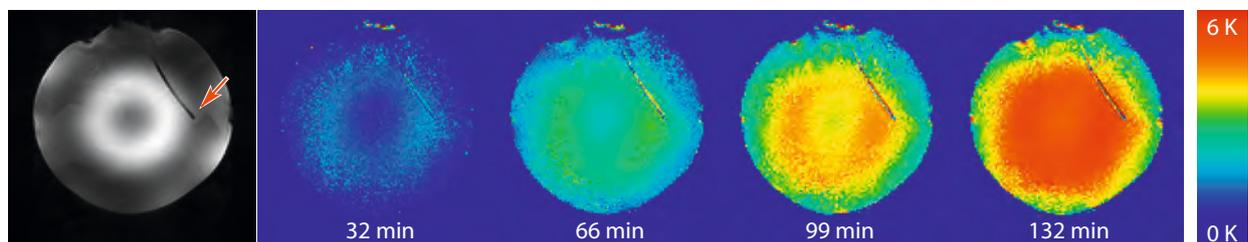
Figure 4.1.7.1 An axial phantom water magnitude image and successive temperature maps (acquisition times below each figure). The red arrow indicates the tip of temperature sensor 2.
