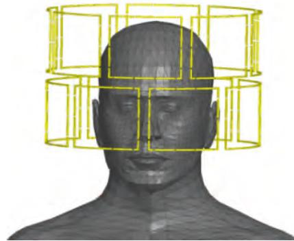
Figure 4.3.4.1 9.4T array geometry setup. Only radiative elements and human model are shown.
