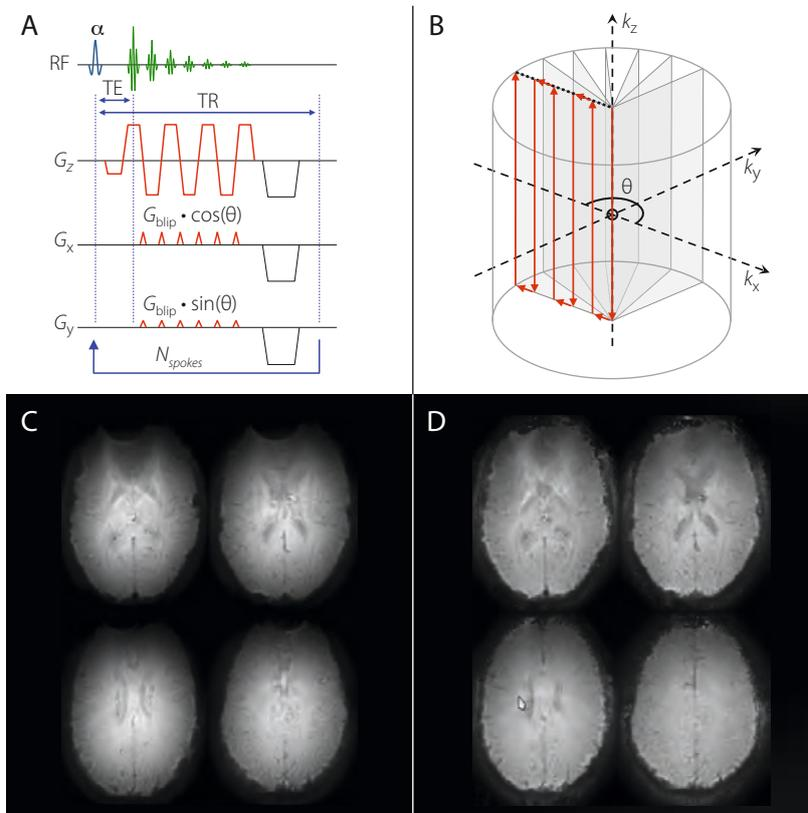
Figure 6.1.2 Schematic pulse sequence diagram (A), sampling trajectory of a single spoke in the cylinder of acquired  $k$ -space data (B), and phase-corrected images recorded from a healthy volunteer ( $\alpha$  24°,  $TE/TR$  2.8/95 ms, 1.5-mm isotropic voxels) without (C) and with (D) multi-frequency distortion correction.
