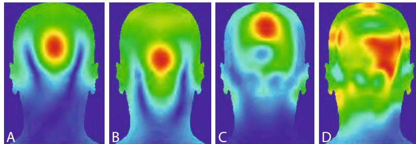
Figure 4.3.4.4 Tuning condition for displacement "26 mm". (A) and (B)  $B_1+$  slices rescaled to individual maximum, (C) and (D)  $SAR_{10g}$  slices rescaled to individual maximum; (A) and (C) CP mode, (B) and (D) "+90" mode.
