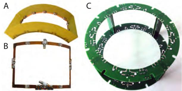
Figure 4.3.1 (A) Single element of an RF transmit coil fabricated with novel printed-circuit board technique. (B) Similar element fabricated by hand. (C) Photograph of a 4-element printed-circuit array.
