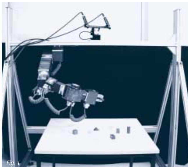
Figure 1: Experimental setup with 6 degree-of-freedom arm and stereo-vision system.
