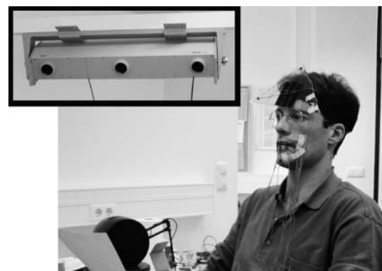
Figure 3: Experimental setup for measuring the lip movements with the Optotrak. The participant is placed in front of the cameras (left-top corner of the picture) with the infra-red Optotrak markers placed on him. Head movement is captured by measuring the position of the three markers on the head-mounted triangle, allowing the computation of the three positional and three rotational coordinates of the skull. Eight markers are used for the lips, which gives a quite accurate representation of both shape and dynamics of labial movements.
