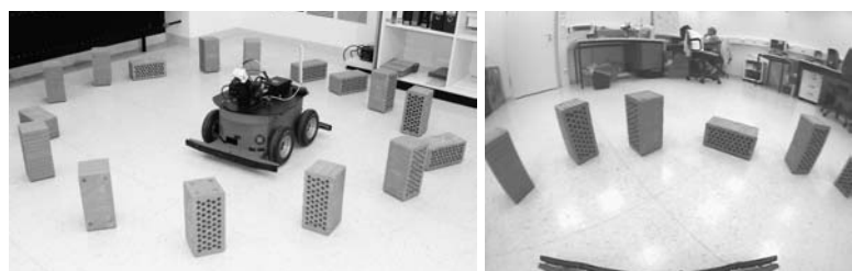
Figure 4: Visually guided mobile robot locomotion: Setup for the collection of training examples (left) and image as seen by the robot's camera, taken from the database (right).
