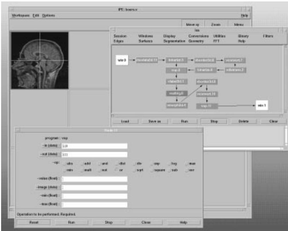
Figure 2. Example view of a processing chain in the visual editor. Individual modules are represented as small buttons whose status is color-coded. The result of a chain is either displayed in a stand-alone viewer or fed back into a workspace window.
