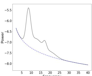
(3) De-trending of the original signal (A) Peak search between 4 – 7 Hz and 7 – 13 Hz and estimation of the peak parameters (B)
