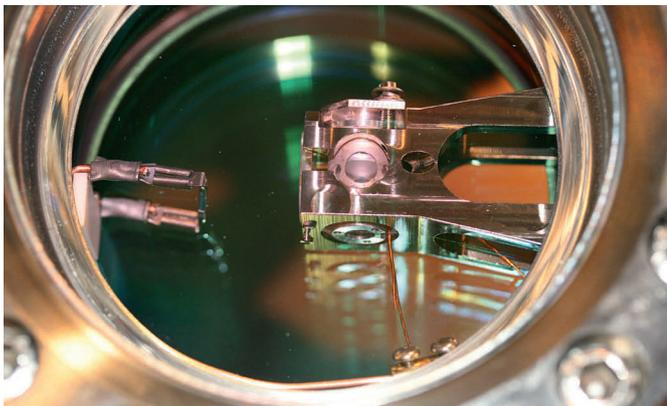
Capturing atoms and photons: Two glass mirrors in the shape of truncated cones are assembled in the stainless steel clasp. One can be seen in this image to the right of center. The Max Planck researchers capture individual atoms between the mirrors. The laser pulses stream into the vacuum chamber through the glass window.
